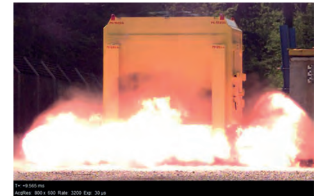
Blast test in an underbelly threat scenario with home-made explosives
