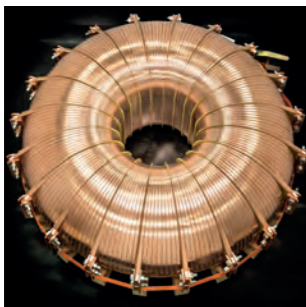
Storage coil of an XRAM generator for the electrical power supply of railguns
