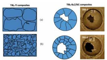
Cracks observed after impact for various samples
