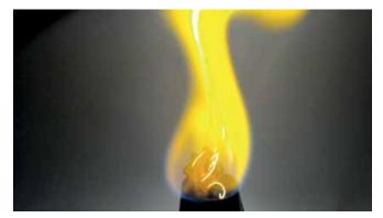
Combustion of propellant grains
