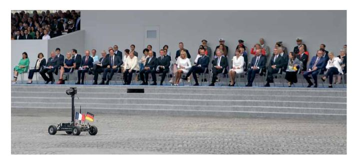
On 14<sup>th</sup> July 2019, ISL's STAMINA-UGV Patrol, carrying the French and German flags, opened up the military parade on the Champs Elysées in front of Emmanuel Macron, Angela Merkel and numerous state representatives. Based on image processing and capable of following itineries without GPS, this smart, cost-effective robot took up a front-line position at this important event dedicated to demonstrating defence innovation capabilities.
