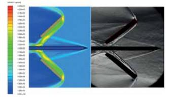
Sabot separation at muzzle exit: simulation (left) and experiment (right)
