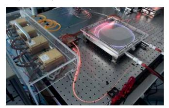
Alignment-free all-fibred laser set-up
