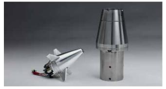
ISL's roll-decoupled guidance module
