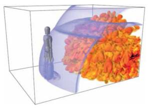
available for the blast threat, such as the Bowen curve and the Axelsson model, can only predict a percentage of lethality when the manikin does not wear personal protective equipment. In order to gain insight into thoracic protective system efficiency against the blast threat, new lung injury tolerance limits have been defined for short duration blast waves. It has been noticed that the chest wall velocity and the intra-thoracic pressure impulse are related to the risk level of lung injury.
