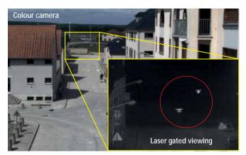
Detection of UAVs using range-gated imaging
