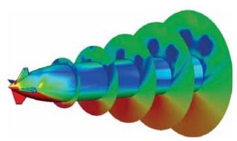
Simulation of the flow around the decoupled fuze guided projectile
