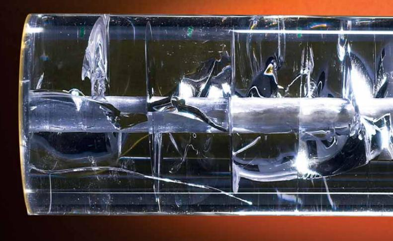
Art and science: the effect of a solvent on a tube used for pyrotechnic tests
