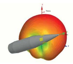
Roll-decoupled 3D radiation pattern associated to a GNSS antenna array
