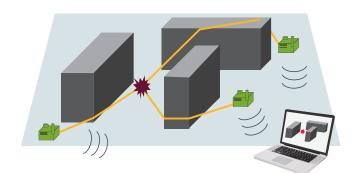
Localisation of an acoustic source (red) in a complex urban environment using a network of distributed sensors (green)
