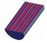
Co-layered propellant charge
