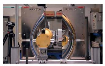
Test-bench to measure transmission and reflection of laser beams
