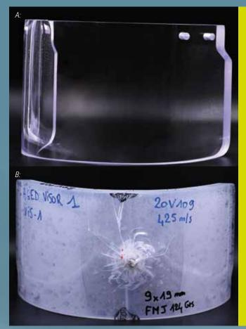
A: Visor in pristine state; B: Visor after ballistic impact
