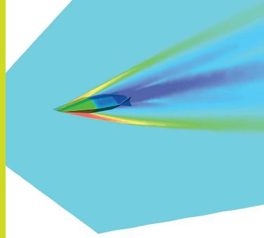
Hypersonic flow computation of ISL-designed, short-range projectile for rapid-fire railgun showing superior low drag performance and directional stability
