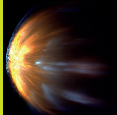
Hypersonic flow field around sphere body in ISL shock tunnel showing influence of generated plasma on radar signature quantified
