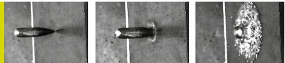
Ceramic plate stops a hard-core bullet calibre 7.62 (frames taken by high-speed camera)
