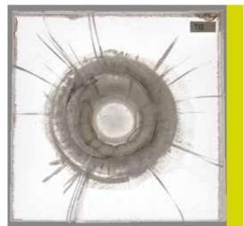
*Composite visor sample after drop tower impact*
