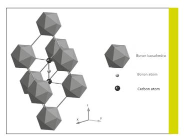
Schematic view of the crystallographic structure of Boron Carbide ( $B_{A}C$ )
