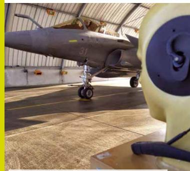
Acoustic tests with specifically developed ISL measurement head on Charles de Gaulle aircraft carrier
