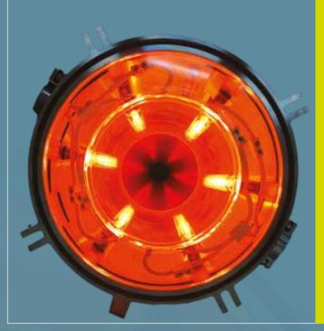
Atomisation chamber of the spray flash synthesis (SFS) process warmed by infrared heaters
