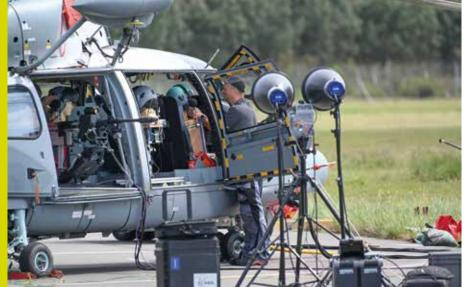
Setting up the shot noise measuring device in a helicopter cabin
