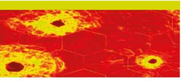
Non-destructive testing image of protective plate after ballistic testing
