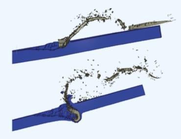
Numerical and experimental investigations on ricochet at impact velocity of 1400m/s against homogeneous armour
