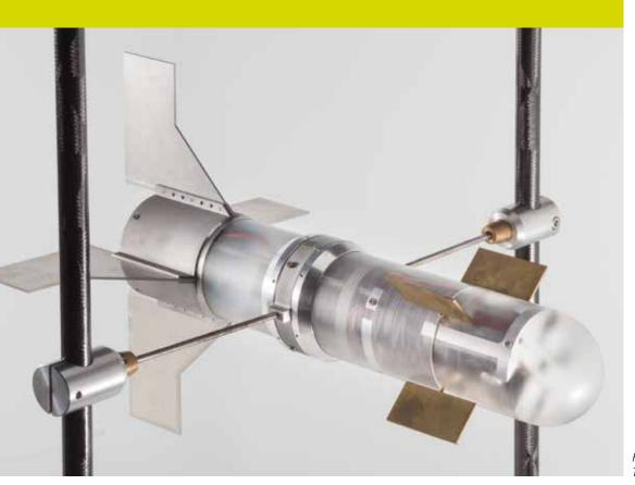
Hardware In-the-Loop (HIL) Wind Tunnel model
