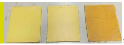
Comparison of aramid helmet composites before (left) and after ageing using different artificial ageing cycles (centre, right)
