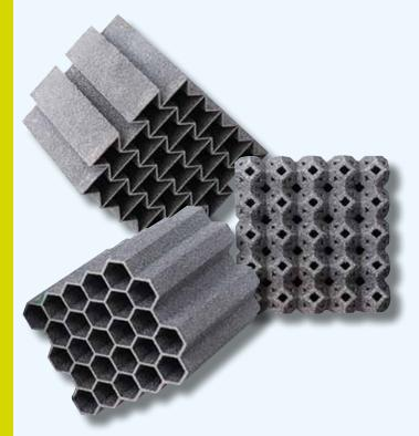
Samples of AlSi10Mg aluminum alloy crushable lattice additively manufactured by Direct Metal Laser Sintering
