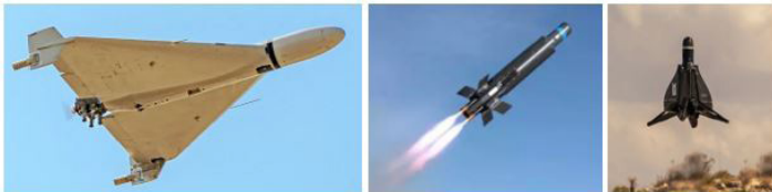
HESA Shahed-136 loitering munition (left), Raytheon Coyote Block II "missile-like" drone (middle), Anduril Roadrunner VTOL drone (right).
