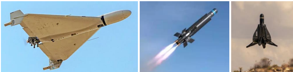
Figure: drone suicide HESA Shahed-136 (gauche), drone-missile Raytheon Coyote Block II (milieu), Anduril Roadrunner VTOL drone (droite).
